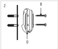
Attach the retractable line case to the fixed bracket.
