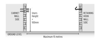
2. In cabinet wall side, turn mounting bracket facing against the wall and mark two hole positions.
