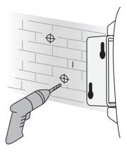
3. In retaining hook wall side, drill hook position with 8mm diameter x 35 - 40mm depth. (For Twin Line model, repeat Step 3 to drill second hook position. Recommended centre to centre hole positions 50mm - 80mm.)
